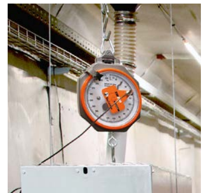
Use of the dial-type crane scale
