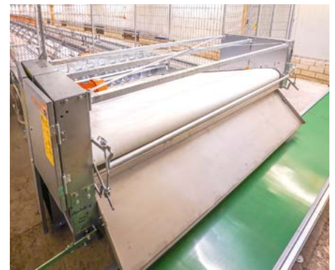
The manure is transferred to a floor-level cross belt
