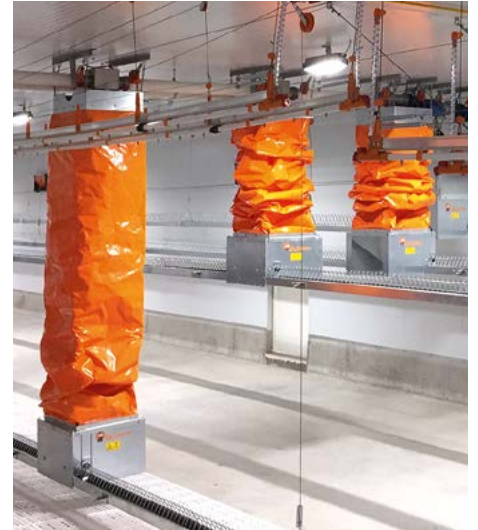
Feed hose: space-saving and convenient
