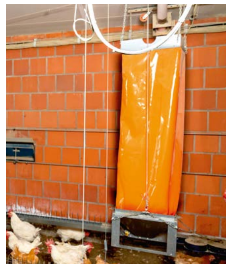
Feed hopper with foil hose
