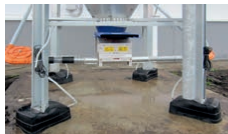
Cover for silo foot for accurate weighing even in extreme weather
