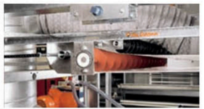
Manure belt idler roller with cleaning auger (option), removes dust and feathers from the returning belt
