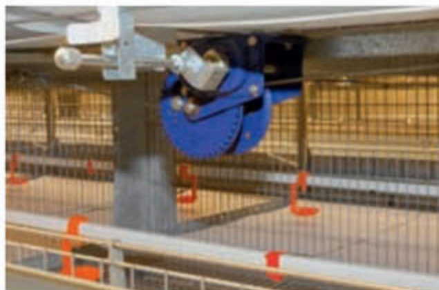
Centrally installed winch to adjust the height of the drinker line
