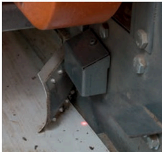
Light sensors monitor the belts
