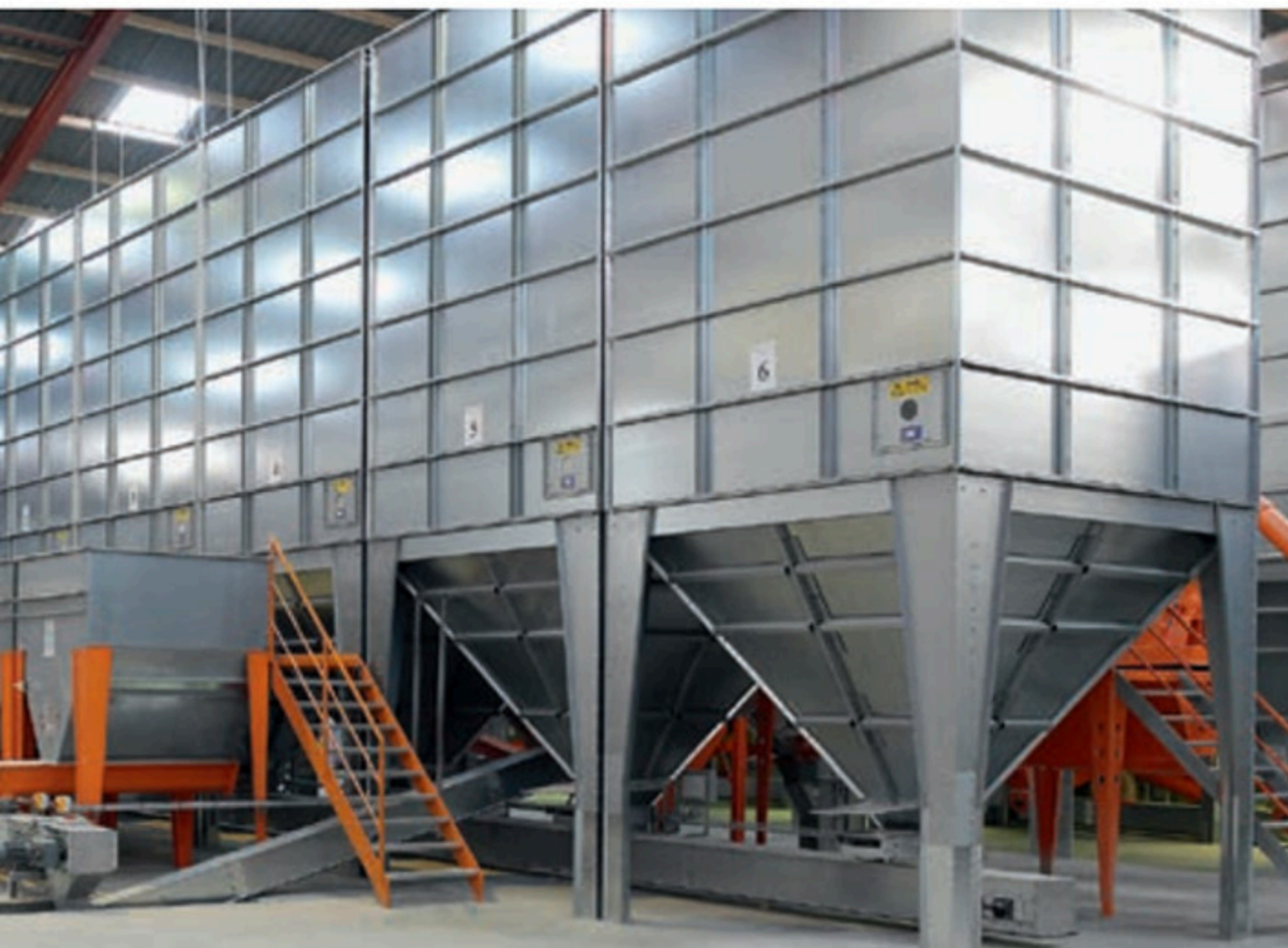
Indoor silos for storage of completed mixes
