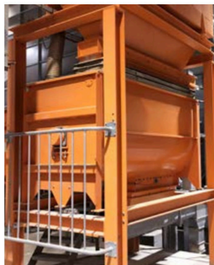
Horizontal mixer with preliminary holding bin
