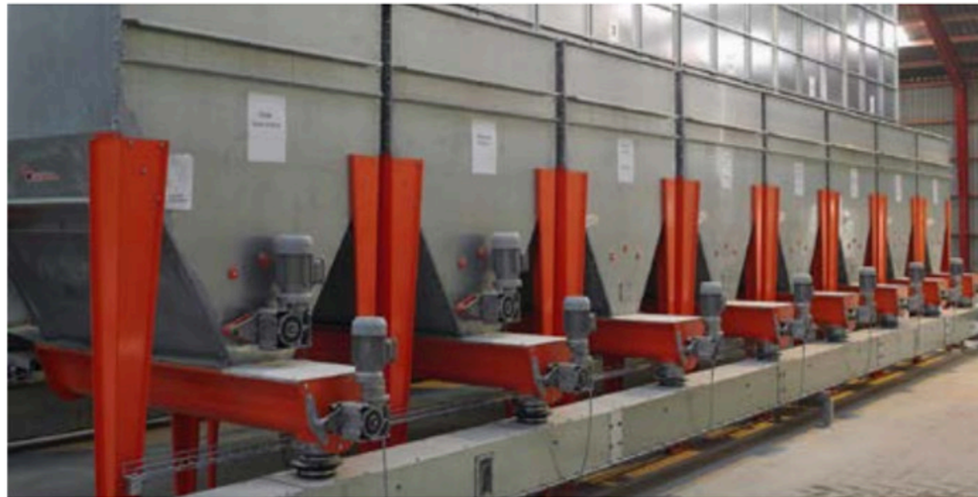
Hoppers, each with a capacity for up to 2 t minerals
