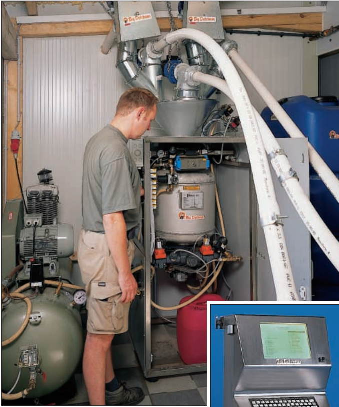
Pre-assembled feed unit with high-pressure tank made of stainless steel
