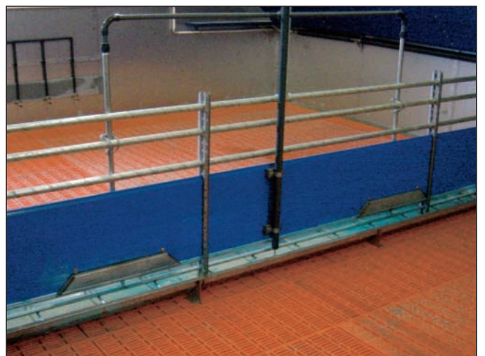
Sensor trough made of stainless steel with trough dividers
